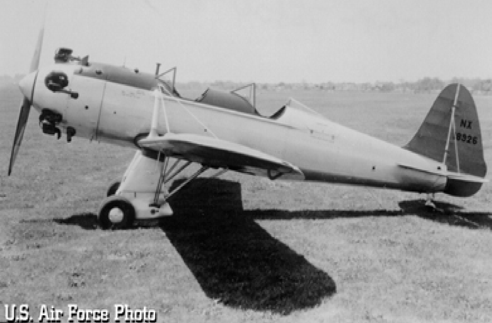
Ryan PT-22 with a Kinner radial engine
